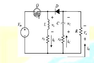
Fig.11: DC-DC Buck Boost converter circuit diagram
